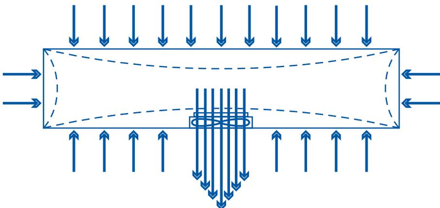
Negative pressure only works efficiently if the house is effectively sealed. In a house that is effectively sealed against air leaks, all the air entering the house comes in through the desired air inlets and uncontrolled air leakage will be minimized.
