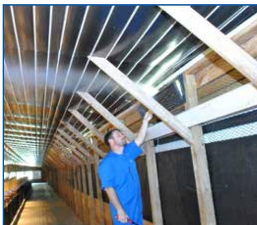
When smoke testing a house, it is advisable to do it under worst-case conditions, that is, when the house is at brooding temperature and when the ambient temperature is at, or close to, as cold as it may get. As long as all air inlets are opened an equal amount the smoke test can be completed on any inlet. Hold the smoke bomb approximately 5-10 cm (2-4 in) below or away from the inlet or curtain opening to allow a sufficient volume of smoke to be emitted so direction of flow can be seen clearly.
