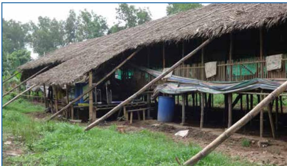
Air flow in open-sided houses is controlled by varying curtain height. Curtains should be fastened to the side wall at the bottom and be opened from the top down as to minimize wind or drafts blowing directly on the birds.
