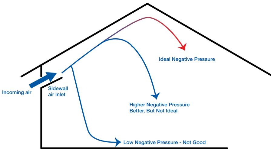
A high air speed will also ensure good mixing of the cold incoming air with the warm in-house air that collects in the apex of the house (**Figure 105**), making the incoming air warmer and reducing its relative humidity allowing it to absorb moisture.
