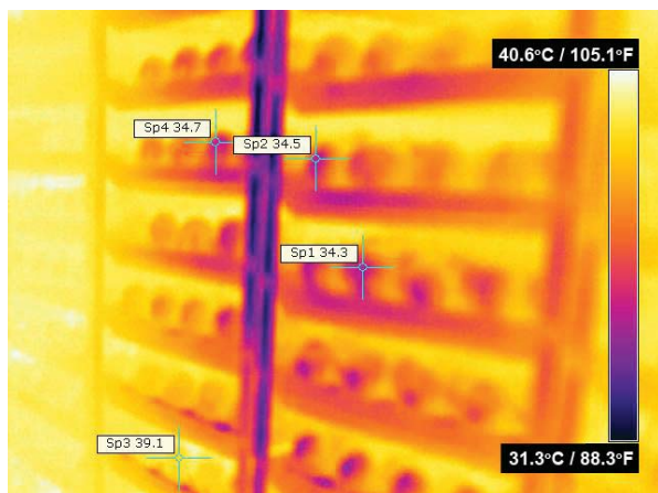
Figure 3: Thermal camera picture showing wet and cold eggs caused by poorly maintained humidity nozzles.
