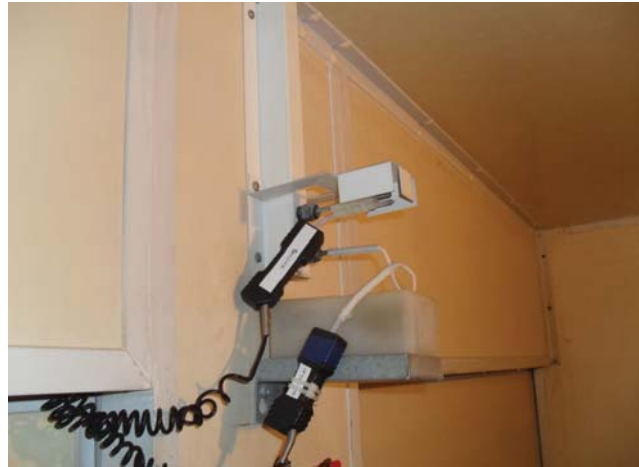
Figure 7: Calibrating by locating the calibration probe next to the machine temperature sensor.
