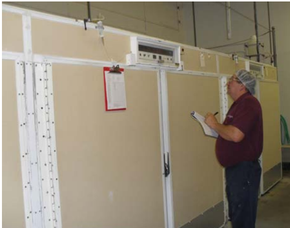
Figure 2: Check and record the setter and hatcher environment several times during the day.
