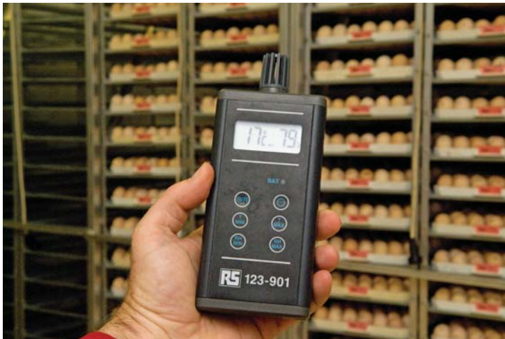
Figure 11: Checking egg store environment using a temperature and humidity sensor.
