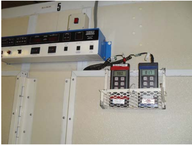
Figure 7: Calibrating by locating the calibration probe next to the machine temperature sensor.
