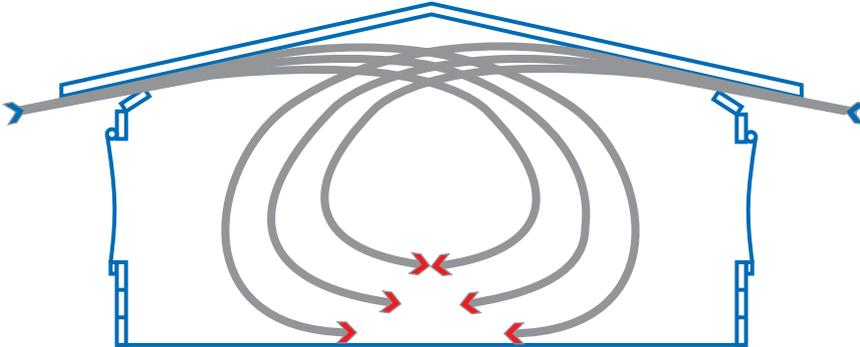
Where the ceiling has structural obstructions crossing the path of the airflow, it will be necessary to fit the air inlets with direction plates so that the incoming air can be directed below the obstruction, but still to the peak of the roof (**Figure 107**). Without direction plates, the incoming cold air will be deflected down onto the birds.
