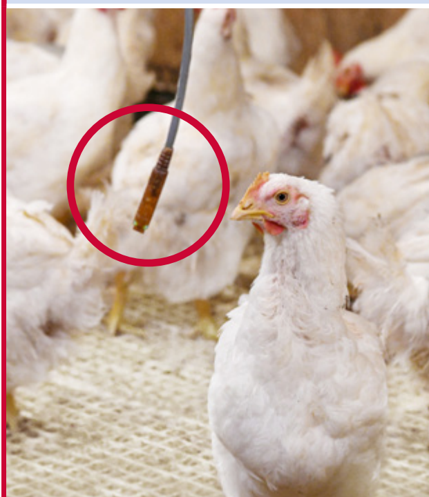
Figure 17 Correct location for temperature/humidity sensors.
