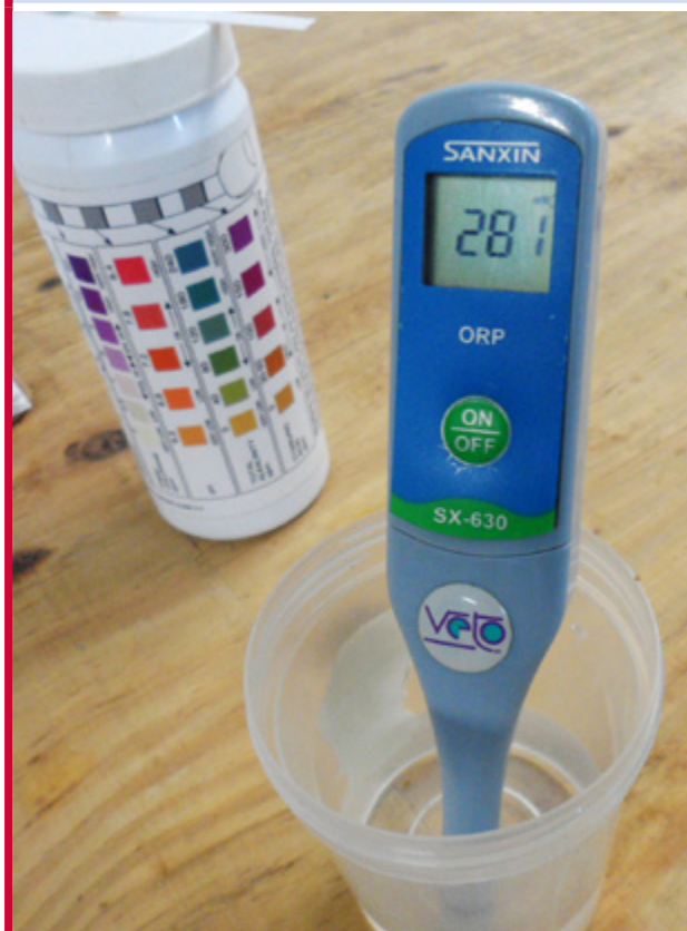
Figure 122 An example of an ORP meter.
